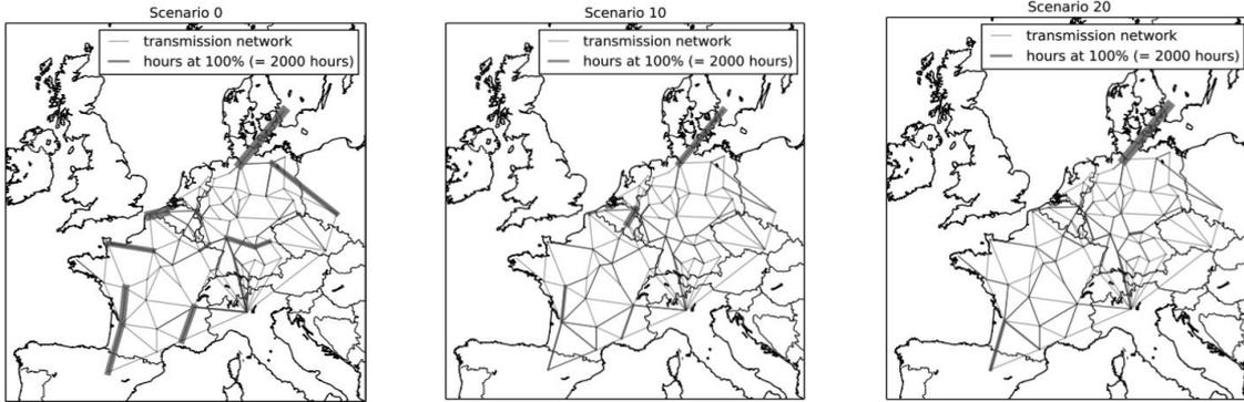
Figure 6: Line load after redispatch measures in different scenarios 2030
