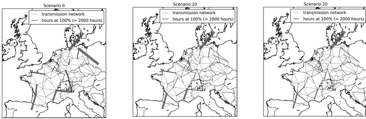
Figure 5: Line load after redispach measures in different scenarios 2020
