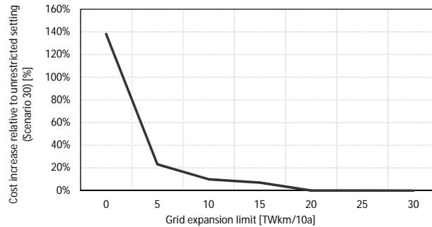
Figure 7: Total system cost decrease with grid expansion
