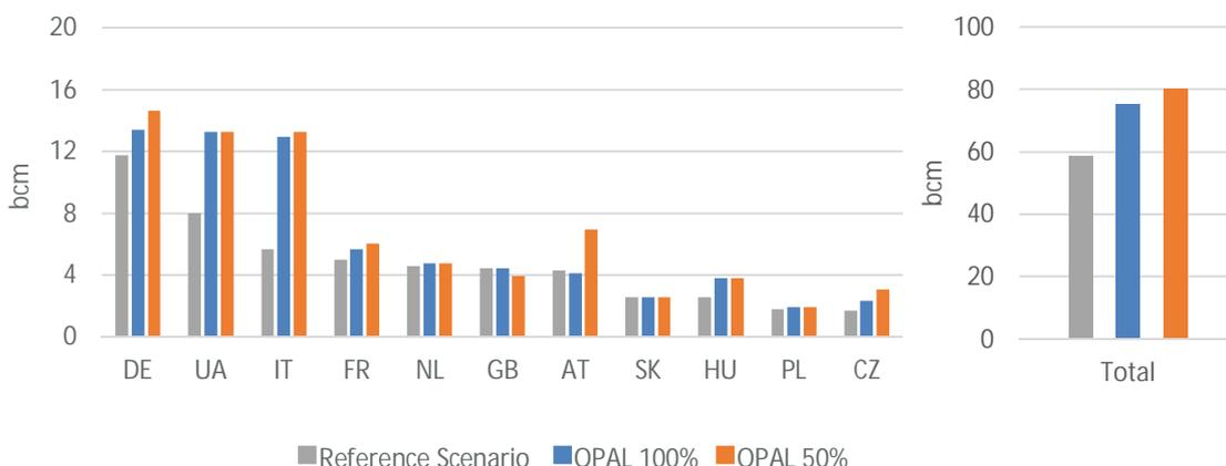
In the case of pipeline transmission, several limitations configure the redistribution of flows between both scenarios. They are represented in Map VII. Figures show transit during the 6 month duration of the scenario. The numbers to the left represent figures for the OPAL 50 scenario while the figures to the right represent transmission on the OPAL 100 scenario. Exceptionally, OPAL's capacity represent full year volumes (16 bcm/y and 32 bcm/y under a TPA exception).
